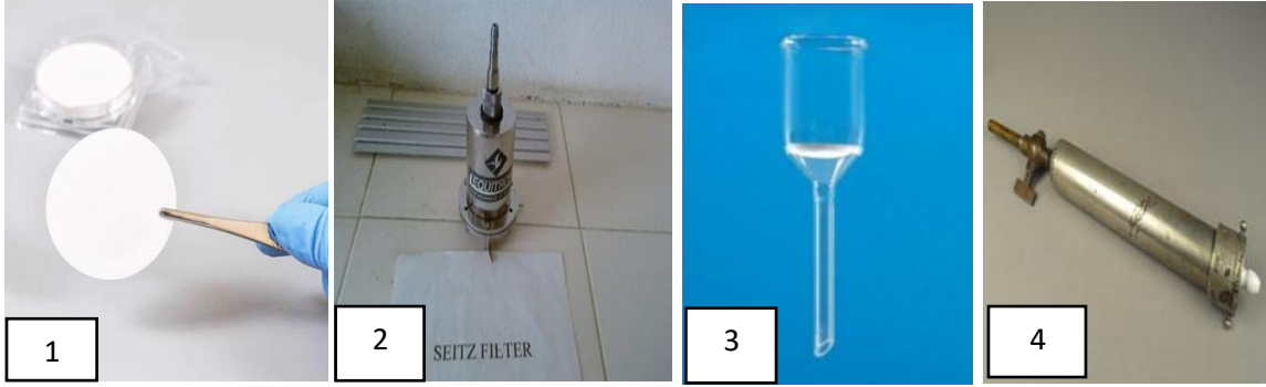
1- Membrane filters, 2- Seitz filters, 3- Sintered glass filter, 4- Chamber land filters
